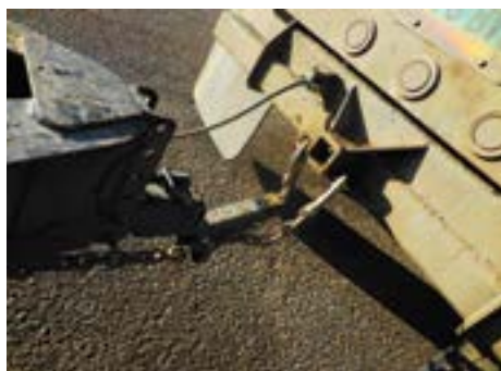
A detached trailer due to improper receiver hitch (bumper hitch). Photo by John Watkins MCS54.
