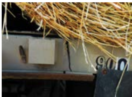
Cracked fifth wheel upper plate with spreading of the trailer frame. Photo by John Watkins MCS54.
