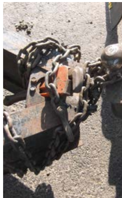
Broken pintle hitch missing locking latch. Photo by John Watkins MCS54.
